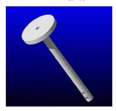
When inserted in a standard plastic lined Tee, our PTFE Injection or Mixing Tee nozzles allow injection of acid, or any difficult-to-handle fluid, into the fluid stream of your system. Our solid PTFE nozzles are optimized for uniform dispersal into the system and are available for 1" to 8" sizes for standard and reducing tees. Also available in PVDF and Polypropylene.
