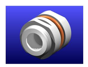
To maximize creep resistance, FLUOR-O-FLO® PTFE bulkhead fittings (and all female FLUOR-O-FLO® fittings) are made from Micromold's MICROFLON<sup>TM</sup>, a special virgin PTFE. PVDF fittings are made from natural virgin materials. Standard fittings are supplied with Teflon® FEP encapsulated, hollow core, silicone o-rings.
